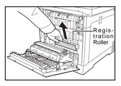
4 If a paper jam does not reach the metal roller as shown, grasp the paper and pull it out.
